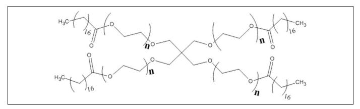
Figure 1. PEG-150 pentaerythrityl tetrastearate (wherein the sum of all instances of n is equal to 150).
