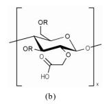
Figure 1. a) structure for Cellulose; b) structure for Carboxymethyl Cellulose Acetate Butyrate, where R represents hydrogen or the acetyl or butyryl moiety.
